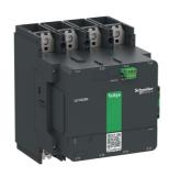
High power contactor, TeSys Giga, 4 pole (4NO), AC-1 <=440V 440A, standard version, 100...250V wide band AC/DC coil
